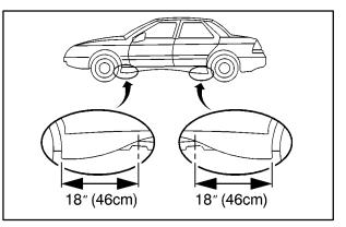
3. Near each wheel well is a notch in the frame which the jack head fits in. The front notch is 9 inches (23 cm) back from the front wheel well. The rear notch is 8 inches (20 cm) forward from the rear wheel well. As is shown in the diagram above, if your vehicle has flared side moldings, both front and rear notches are 18 inches (46 cm) from the wheel wells.
